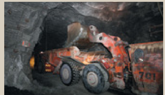
Scoop loads haul truck
