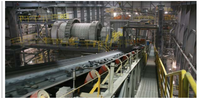
⦿ Ore proceeds along the conveyor in the Process Plant at Snap Lake Mine.
